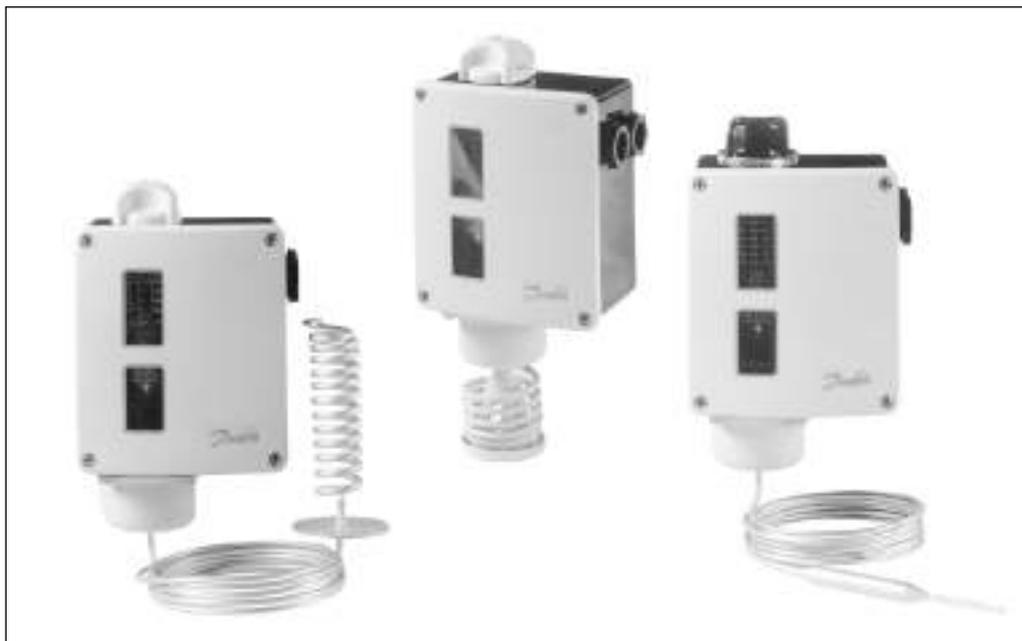
An RT thermostat is fitted with a single-pole changeover switch. The position of the contacts depends on the bulb temperature and the set scale value. The RT series includes thermostats for general applications within industrial and marine refrigeration.
