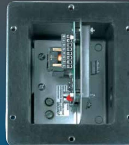
The Model CT Control Unit has a user configurable output relay (using normally closed contacts, normally open contacts or both) which is actuated by either the presence or absence of material. The relay provides a change in contacts as the Probe moves from vertical to tilt and vice versa.
