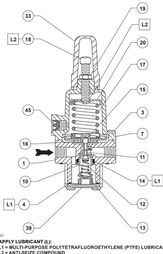
Figure 4. Type 67CS or 67CSR Assembly
