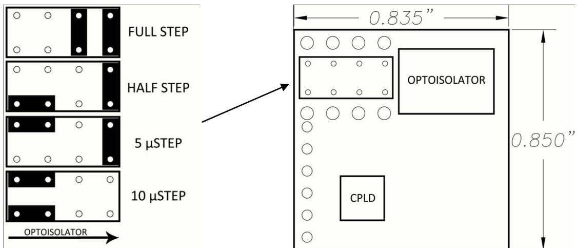
Once the jumpers have been located they may be set according to the diagram below. Please note that the four pins closest to the optoisolator are unconnected and can be used as jumper storage. It is recommended that needle nose pliers or tweezers be used to adjust the jumper settings. The power to the G213V must be turned off before any adjustment is to be made on the step pulse multiplier.
