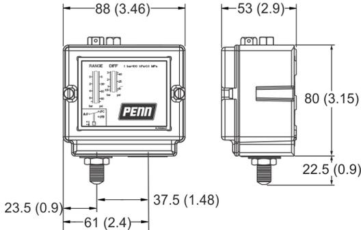
**Figure 2: Capillary connector dimensions, mm (in.)**
